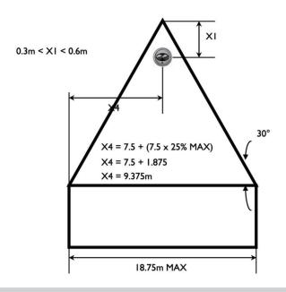
A ceiling or roof with a slope in excess of 4.5 degrees should be regarded as an APEX ceiling / roof.
