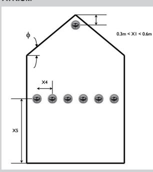
The purpose of this approach is to detect the rising plume rather than the smoke layer. For this approach, supplementary detection using Optical Beam Smoke Detectors close enough to each other to assure intersection of the plume is installed at a level below the lowest expected stratification level.
